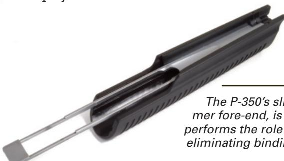
*The P-350's slider, shown here in the polymer fore-end, is a one-piece component that performs the role of dual action bars, virtually eliminating binding in the pump gun's action.*
